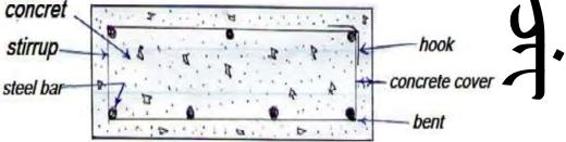
Through the figure, the reinforcement is usually a group of straight bars and loops (stirrups). In the case that straight bars of insufficient length overlapping may be needed, and the length of overlap is (25-40 diameter of bar (db) but not less than 300 mm.
